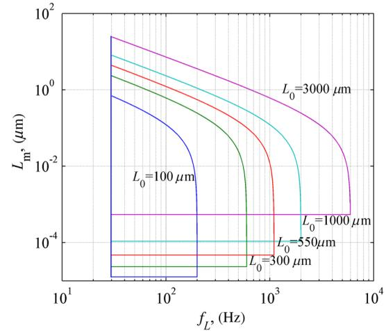
Fig. 2 Limits of the amplitude and frequency of the harmonic baseline variation for different baseline values.
