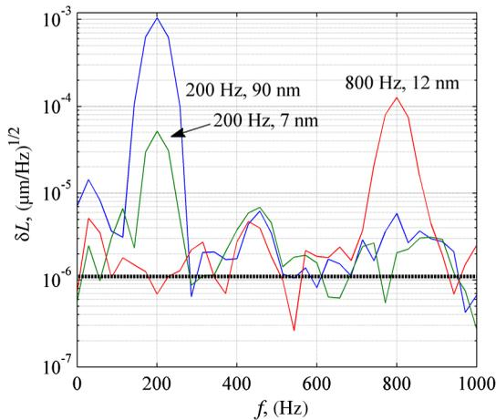
**Fig. 4** Spectral density of the measured baseline oscillations for  $L_0 \approx 550 \mu\text{m}$  (solid lines), noise spectral density estimated according to Eq. (20) (dotted line).
