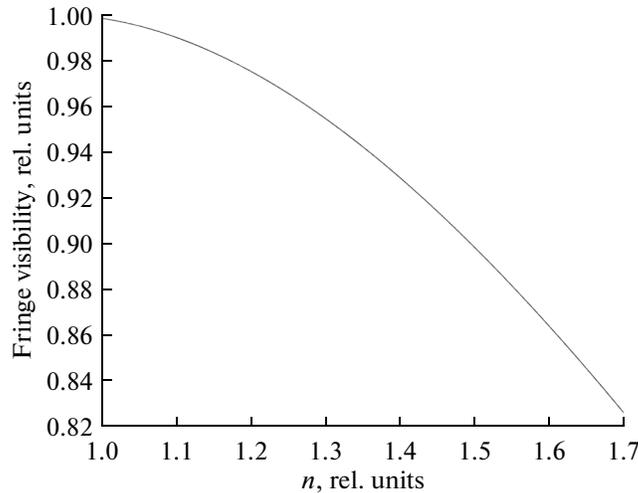
**Fig. 2.** Calibration curve of the interferometer spectrum fringe visibility and the refractive index of the media at the right side of the Si plate.
