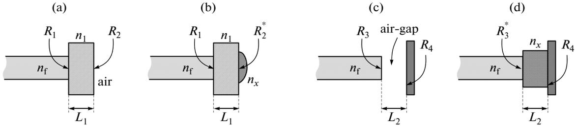
Fig. 1. Interferometers, used for finding the refractive index and the absorption of the investigated media.
