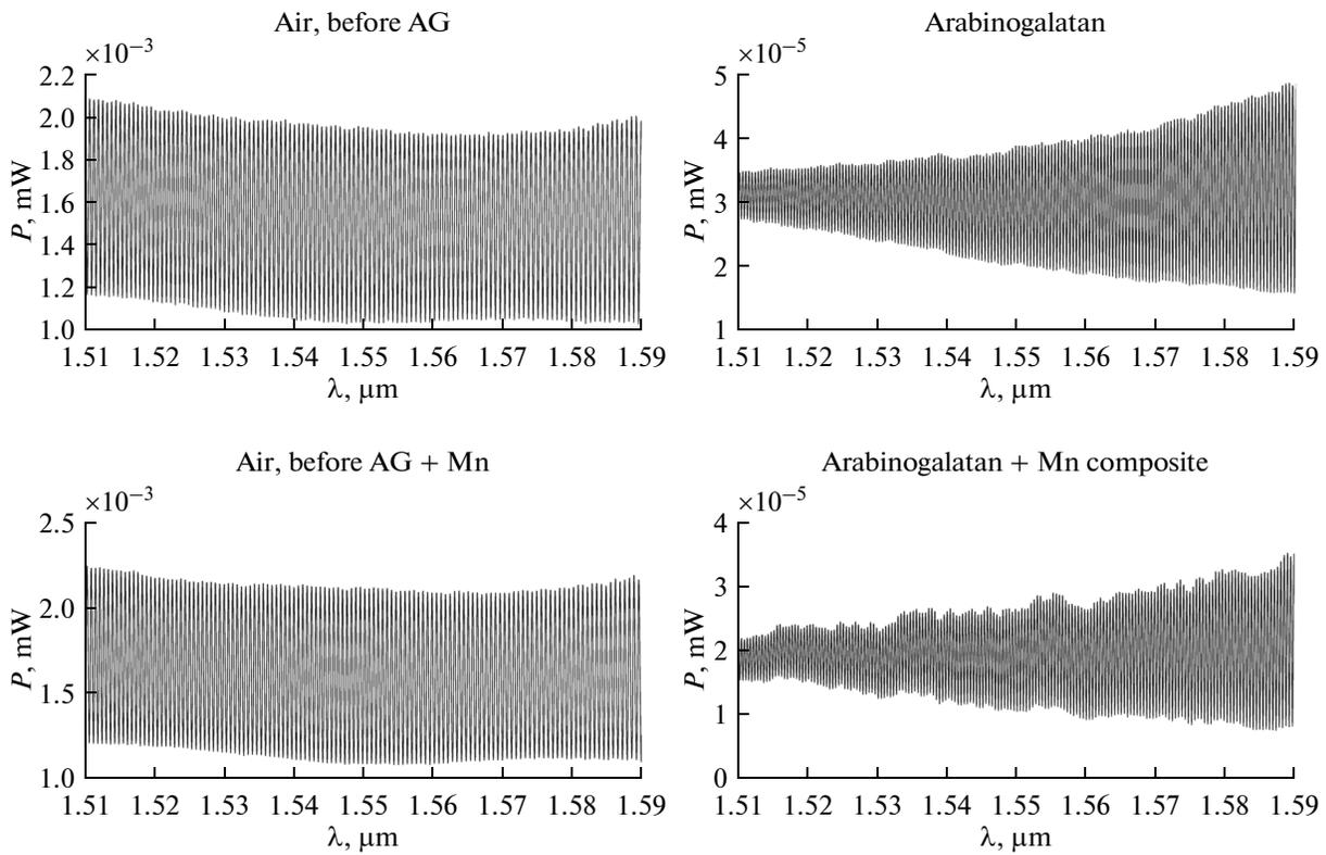
**Fig. 4.** Spectral functions of the interferometers with air, AG and Ag + Mn particle composite.
