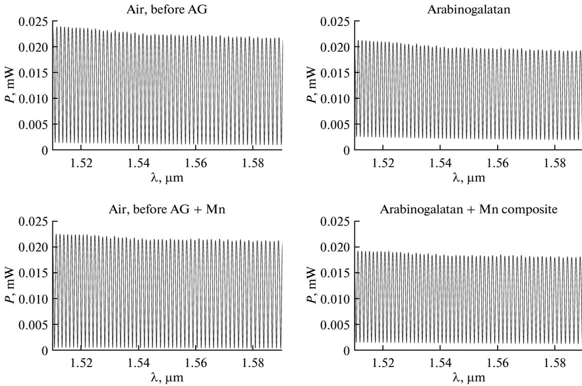
**Fig. 3.** Spectral functions of the reference Si-plate interferometer with air, AG and AG + Mn composite on the right side of the plate.
