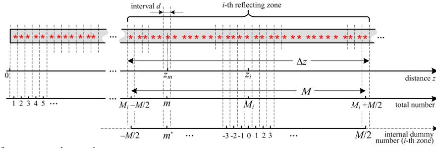
Fig. 2. Relative positions of scatterers and scattering zone.
