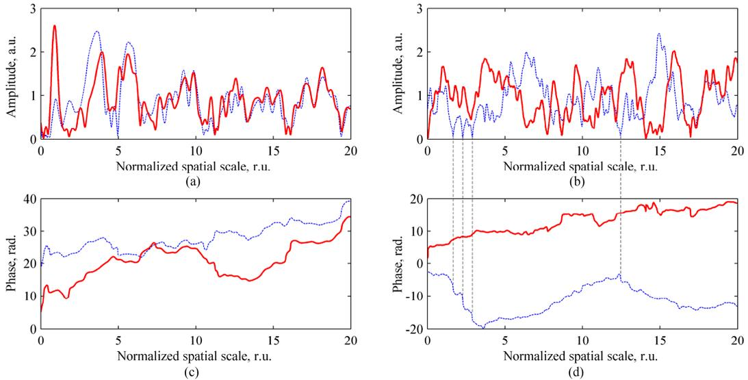
Fig. 4. Comparison of spatial dependencies of amplitude and phase of two realizations of experimental (left plots) and simulated (right plots) backscattered waves (r.u., relative units). Solid line: first trace in data set; dotted line: trace acquired 10 s later. Some of the amplitude fading points and corresponding phase jumps are highlighted by vertical lines.
