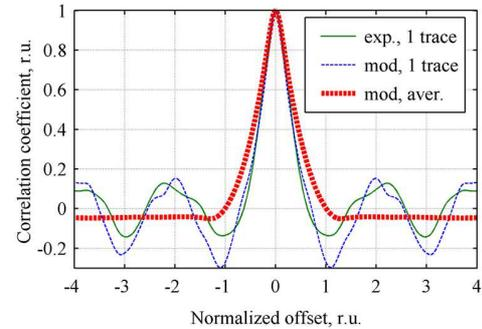
Fig. 7. Autocorrelation functions of amplitude traces: single realizations (experimental, thin solid line; simulated, thin dotted line; simulated signal averaged over 2000 realizations, thick dashed line),  $T_p = 90$  ns.
