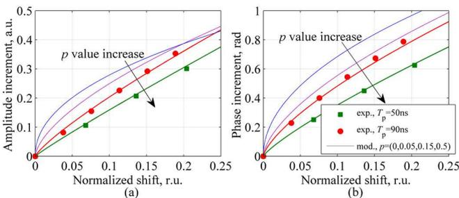
Fig. 8. Relation of differentiated amplitude and phase rms and the length of differentiation interval. (a) Amplitude. (b) Phase. Solid curves illustrate modelling results with different pulse shapes; round dots are experimental results for 90-ns pulse; square dots are experimental results for 50-ns pulse.
