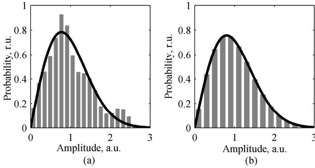
Fig. 5. Comparison of probability density functions of backscattered wave amplitude. (a) Experimental. (b) Simulated. Solid line: Rayleigh distribution fitted to the histogram in each case.
