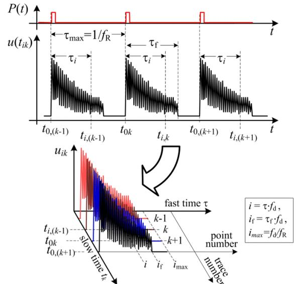
Fig. 1. Demonstration of time-scale transformations in OTDR systems.
