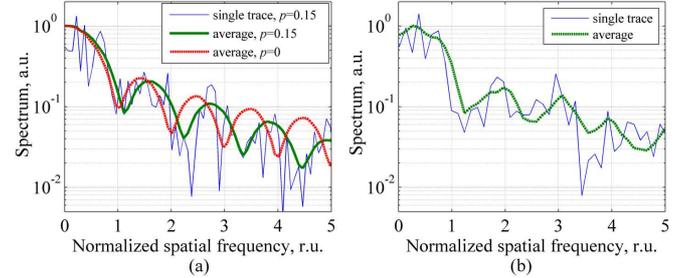
Fig. 6. Comparison of amplitude reflectogram spectra. (a) Simulated data. (b) Experimental data.
