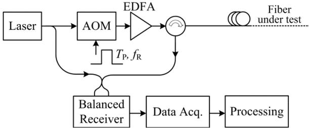
Fig. 3. Schematic illustration of experimental setup. AOM: Acousto-optic modulator, EDFA: Erbium-doped fiber amplifier.
